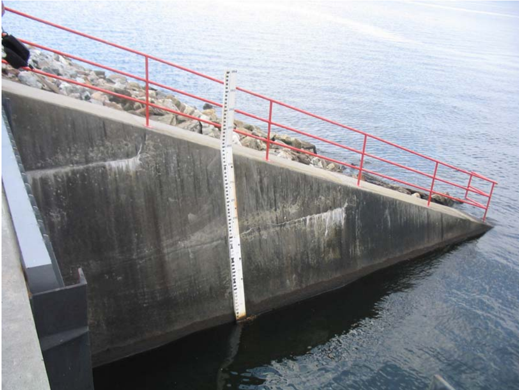
The Gage Used by Dominion at the Dam to Measure Water Height
