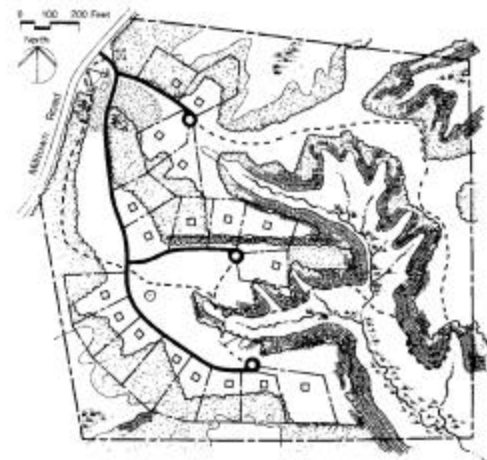
Figure A3-5: Step Five – Drawing in the Lot Lines (Source: Growing Greener )
